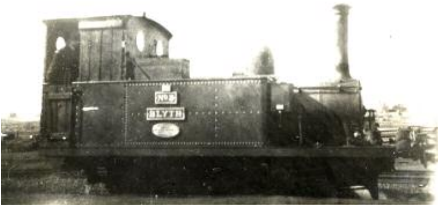
This shot of No.3 "Blyth" is not too sharp but it does show the treatment given to its cab for the winter
