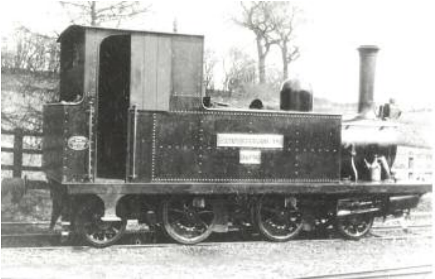
Suffolk winters were often very cold. The cabs of the locomotives offered limited protection. Here No.3 "Southwold" has her cab partially enclosed by extra boarding
